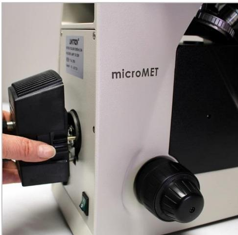
It is fully installed when you feel/hear it snap into place.
