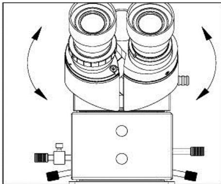
**Fig. 18****Adjusting Interpupillary Distance (Fig. 18)**
