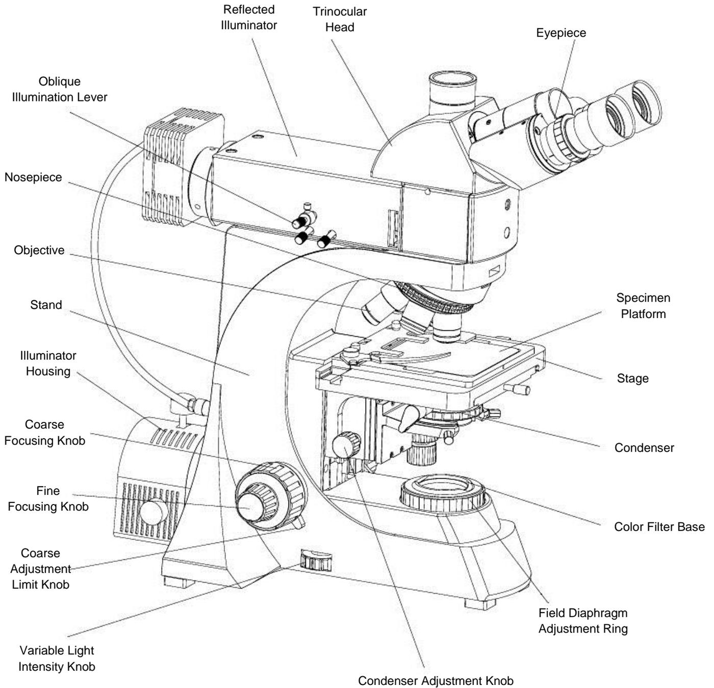
COMPONENTS DIAGRAM 4 – Reflected & Transmitted Model
