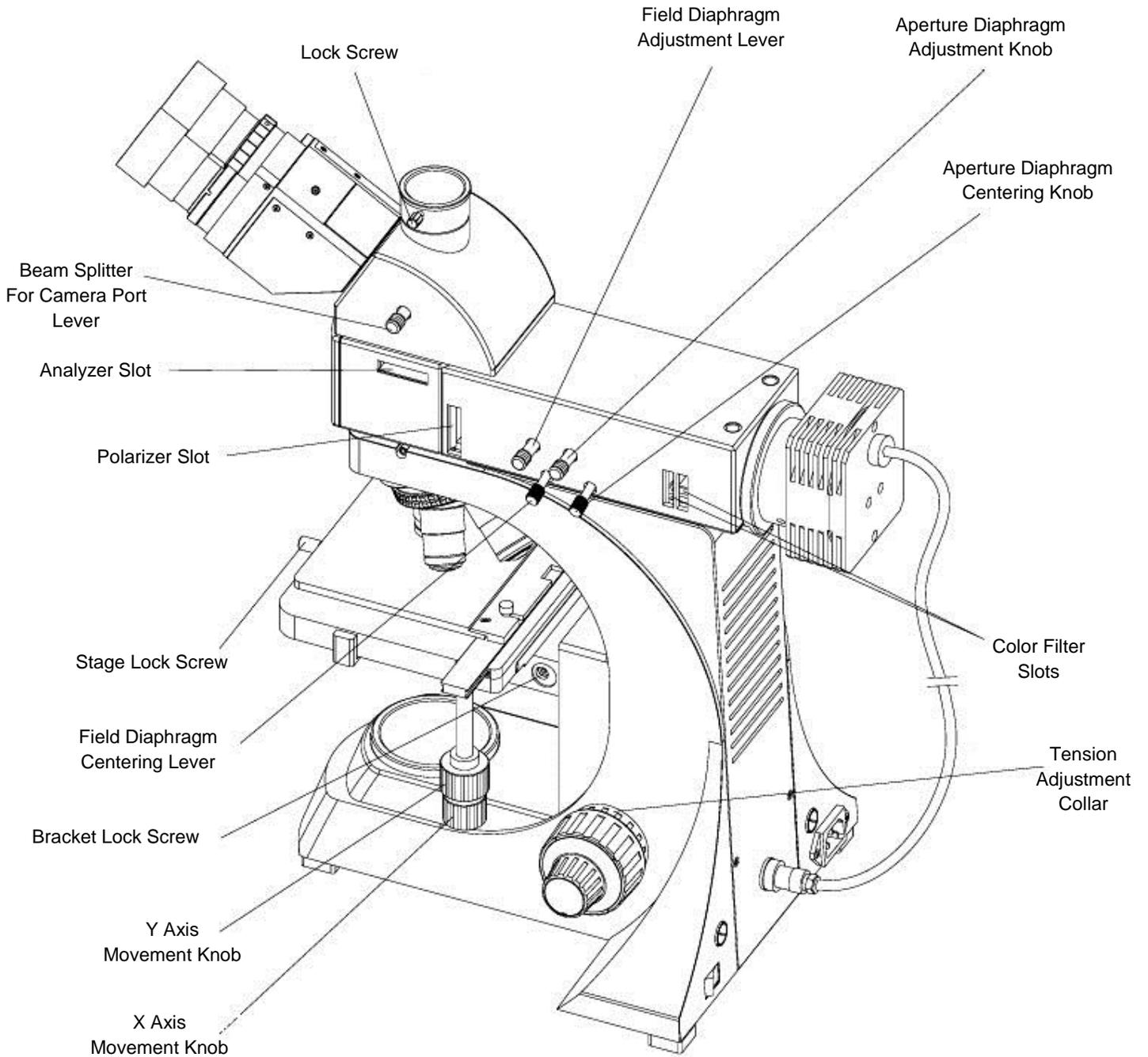
**COMPONENTS DIAGRAM 3 – Reflected & Transmitted Model**
