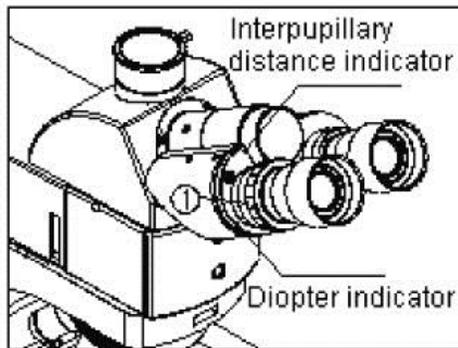
**Fig. 17****Adjusting the Diopter (Fig. 17)**
